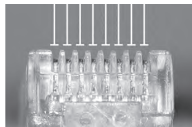
Contacts properly seated (flat crimping).
