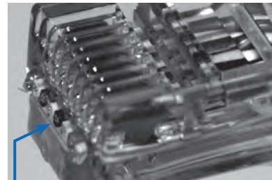
Contacts were not correctly cut off - will prevent proper seating in socket.
