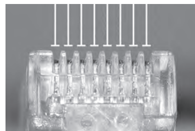
Contacts properly seated (flat crimping).
