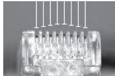
Contacts not seated properly (bowed crimping).
