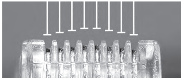
Figure 1.9b: Contacts are not seated properly.
